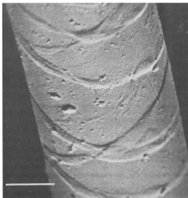
Figure 2 Typical surface banding of the inner surface of a Kevlar 49 fibre loop. Scale marker 4 \mu\text{m}
